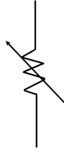
Figure 3. The circuit symbol for variable resistors is presented. This symbol is used throughout this paper to represent both thermistors and potentiometer.
